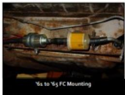
FC vehicles have an easy install along the vertical member just to the rear of the tank where the steel line connects to the rubber hose from the tank; also lots of room for a larger, see through filter.
